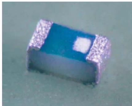
Photo 1: High Q-type chip coil from the LQP03T series
