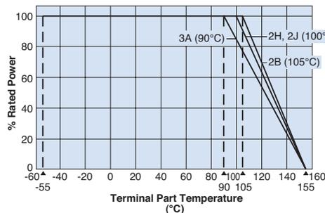
For resistors operated terminal temperature of described for each size or above, a power rating shall be derated in accordance with the derating curve above. Please refer to "Introduction of the derating curve based on the terminal part temperature" on the beginning of our catalog before use.
