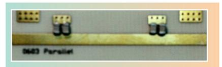
▲ Figure 9 Test fixture of Figure 3 populated with closely spaced 0603 (600S) capacitors.
