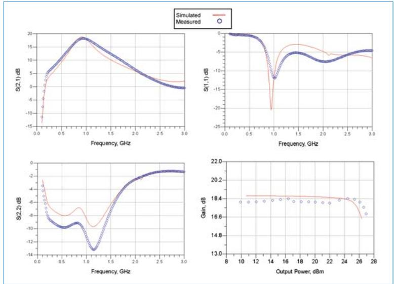
**FIGURE 4** Results from S-parameter and gain compression measurements compared to model-enabled simulations. Note the shift in the input return loss. The 50 ohm power sweep frequency is 900 MHz.
