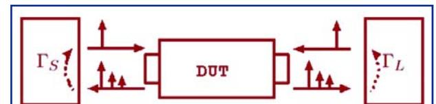
Figure 2: Source and Load Mismatch Effects
