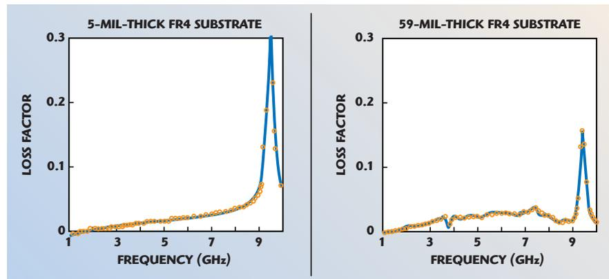
▲ Fig. 3 Forward (solid line) and reverse (circles) loss factor measured on a 5.6 pF 0603 capacitor.
