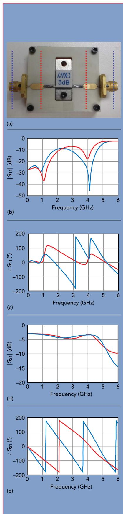
▲ **Fig. 2** Comparing reference plane measurements of a 3 dB attenuator on 60 mil Rogers 4003C (a).  $|S_{11}|$  (b),  $\angle S_{11}$  (c),  $|S_{21}|$  (d) and  $\angle S_{21}$  (e).
