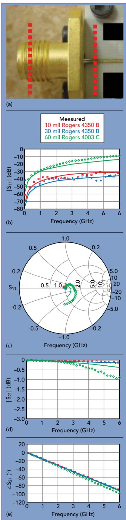
▲ **Fig. 1** Measured vs. modeled (solid lines)  $S$ -parameters for the feed-thru configuration (a) using several Rogers substrates.  $|S_{11}|$  (b),  $S_{11}$  (c),  $|S_{21}|$  (d) and  $\angle S_{21}$  (e).
