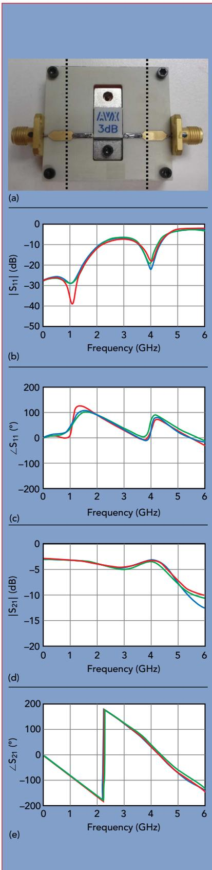
▲ Fig. 3 Comparison of measured and modeled S-parameters of a 3 dB attenuator (a).  $|S_{11}|$  (b),  $\angle S_{11}$  (c),  $|S_{21}|$  (d) and  $\angle S_{21}$  (e).
