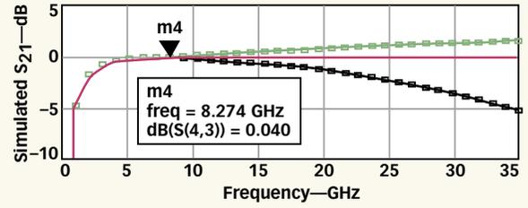
3. These simulated  $S_{11}$  responses for an ideal capacitor (thick black line), equivalent circuit model (magenta circles), and as extrapolated from a data set truncated at 6 GHz (blue squares).
