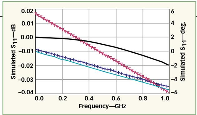
8. These plots show low-frequency extrapolation of HEMT  $S_{11}$  data from a 2-to-26-GHz data set (red triangles = magnitude, blue circles = phase) compared to equivalent-circuit simulations (bold black line = magnitude, green line = phase).
