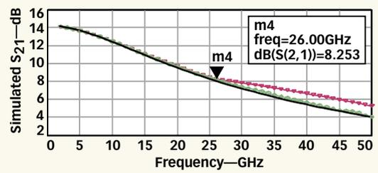
6. These plots compare  $S_{21}$  simulations for frequency extrapolations from the 26-GHz data set (red triangles) and the equivalent-circuit model (bold black line) to the 50-GHz data (blue circles).
