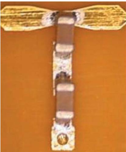
▲ Fig. 4 Shunt-series capacitor configuration.
