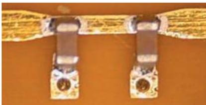
▲ Fig. 3 Shunt-parallel capacitor configuration.
