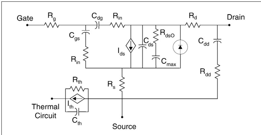
Figure 2 · Topology used in the CMC model.
