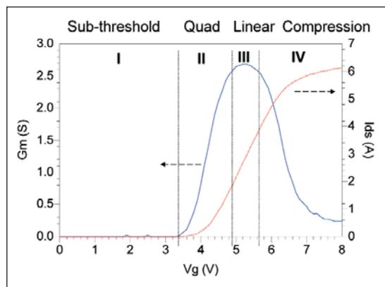
Figure 1 · Four region current behavior of the 1 watt LDMOS cell device used in this development.
