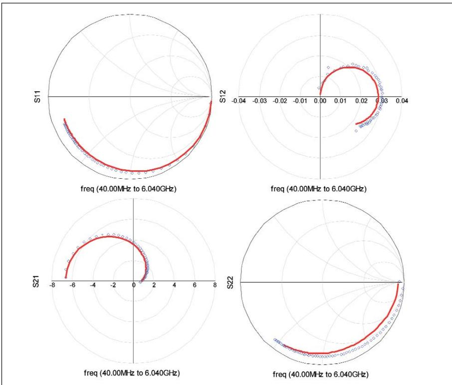
Figure 5 . Small-signal simulation for the 1 watt LDMOS cell. Displayed is measured S-parameter data (Blue circles) and an Agilent ADS simulation of the CMC model (Red line) at  $V_{gs} = 4.8$  V and  $V_{ds} = 25$  V.
