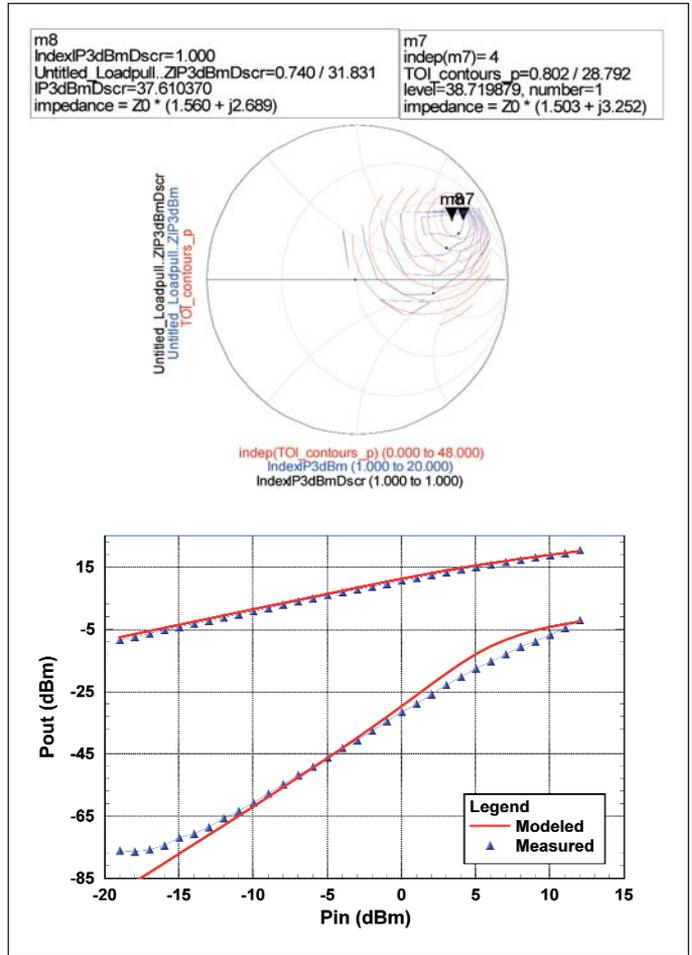
Figure 7 · Displayed are measured IP3 load-pull contours (Blue contours) and the CMC model IP3 results (Red contours) for the 1W LDMOS chip at  $V_{ds} = 27$  V and  $V_{gs} = 4.8$  V with input power ( $P_{in}$ ) is set to 0 dBm at 900 and 910 MHz. The lower graph shows a 2-tone power sweep with the load condition held fixed at the value determined to be optimal from the load-pull simulation.
