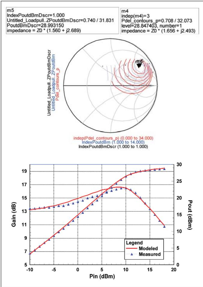
Figure 6 · Single-tone 900 MHz load pull contours are shown in the upper graph. (Blue is measured and Red is simulated data.) The lower graph shows measured and modeled power sweep data for the matching conditions determined from the load-pull simulation.
