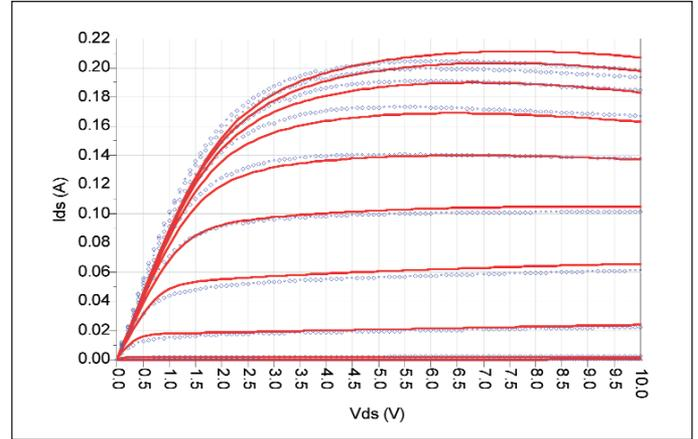
Figure 4 . Forward DC I-V curves for the 1 watt LDMOS cell showing proper treatment of self-heating effects.
