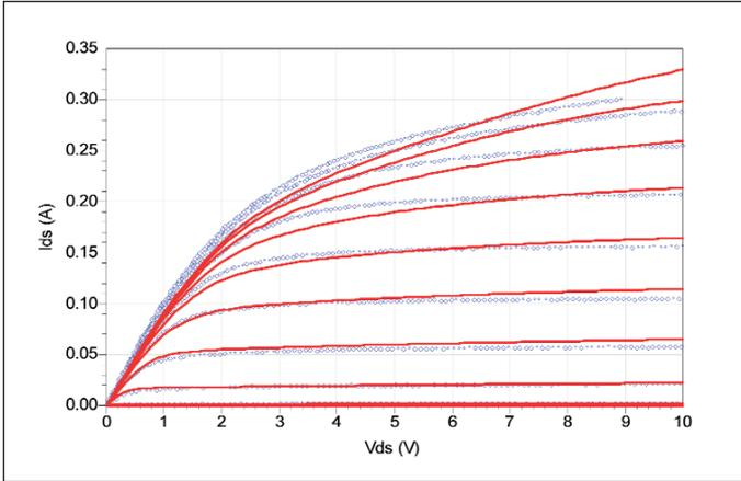
Figure 3 . Comparison of pulsed I-V data from a zero voltage quiescent condition to simulated I-V results with self heating turned off.
