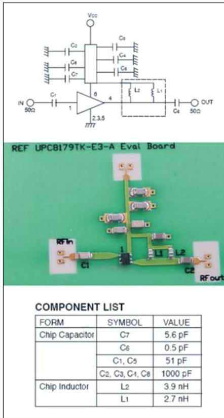
Figure 6 . The NEC UPC8179 2.4 GHz reference validation circuit design used in this work. The circuit was fabricated on a 16 mil Rogers 4003 board. Also shown is the manufacturers recommended component list.
