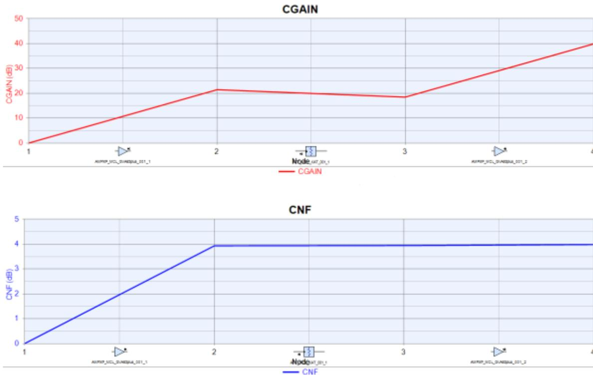
**Figure 3. Simulated cascaded gain (top) and cascaded noise figure (bottom) of the RF chain.**
