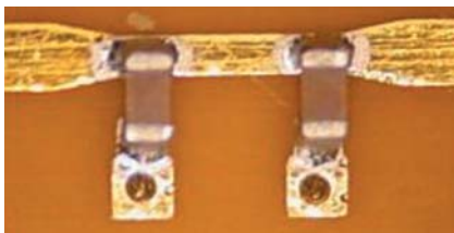
▲ Fig. 3 Shunt-parallel capacitor configuration.
