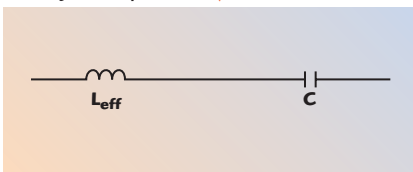
Fig. 1 Simple LC circuit model for a capacitor. ▼
