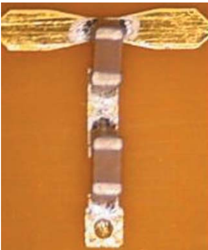
▲ Fig. 4 Shunt-series capacitor configuration.
